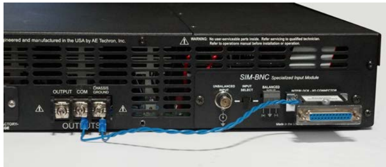
Figure 1 - GCL installed on 7224 amplifier
