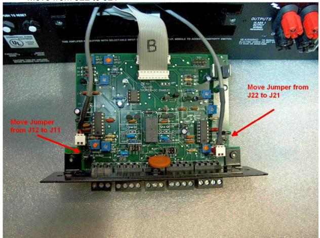
This should Disable the front level controls, without changing the DC Offset of either channel. If you wish to verify the DC offset do the following steps.
