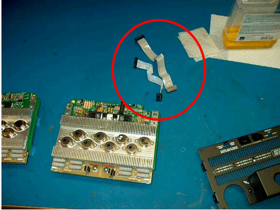
Put the P500/P501 ribbon cables on the working Ch2.
