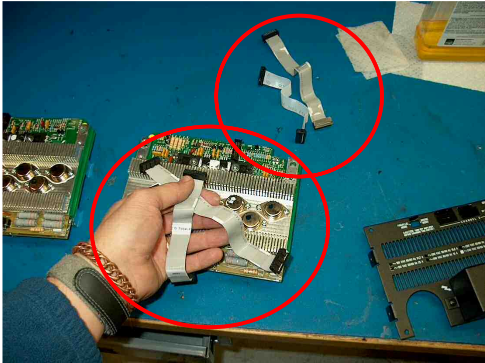
Put the P500/P501 ribbon cables on the working Ch2.
