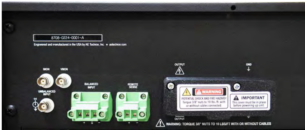
Figure 3.1 – 8700 series I/O Panel (back panel)
