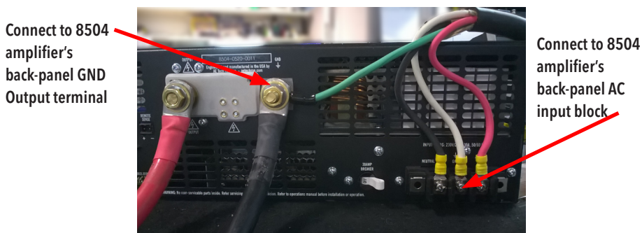
Figure 2 – Connecting to the 8504 Amplifier
