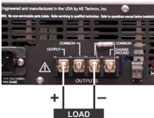
Figure 3.2 – Connecting the Load
