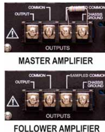
Figure 6.29 – Remove the 2.7-ohm resistor from Follower amplifiers
