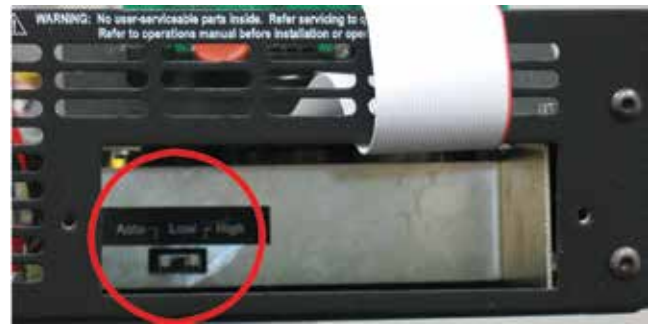
Figure 5.12 – Bi-Level Power Switch Location
