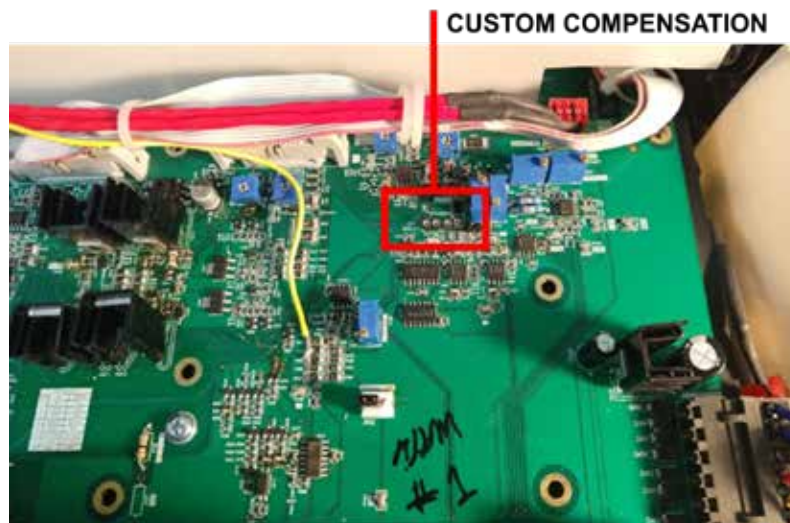
Figure 6.16 – Custom Compensation Component Locations
