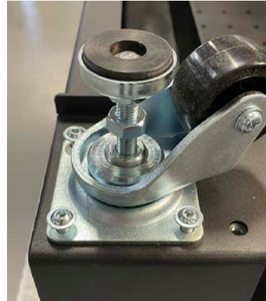
Figure 2.3 – Leveling pads on Cabinet Wheels
