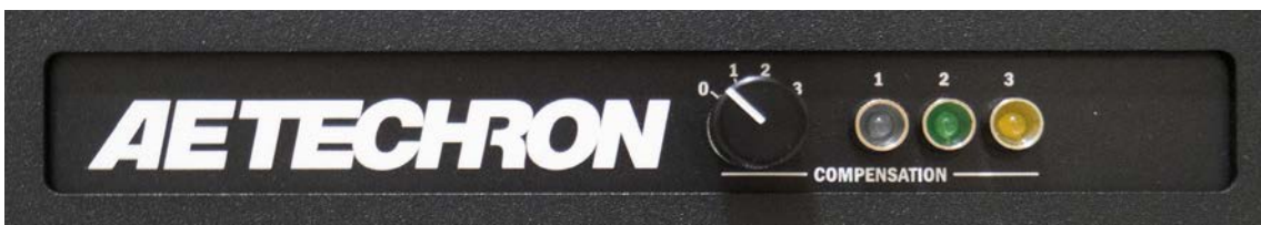
Figure 3.3 – 4301 Compensation Control Panel
