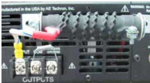
Figure B.2.18 – Connecting the Ballast Resistor
