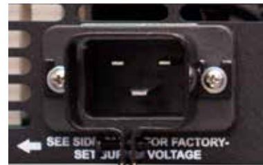
Figure 4.5 – Closeup of AC Mains Outlet
