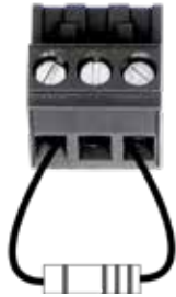
Figure B.2.22 – Terminating the Amplifier Input
