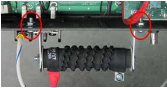
Figure B.2.17 – Mounting the Ballast Resistor
