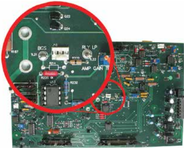
Figure B.1.3 – Configuring Fixed/Variable Gain
