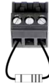
Figure B.2.39 – Terminating the Amplifier Input
