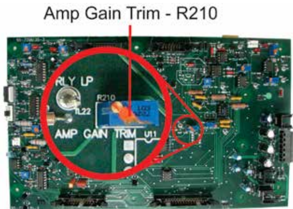
Figure B.2.26 – Amp Gain Trim Location on the Main Board
