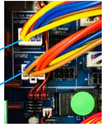
Figure 6.10 – J3 and J7 Plug Locations for High-Current Output
