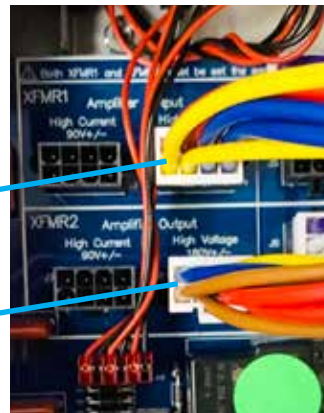
Figure 6.11 – J4 and J8 Plug Locations for High-Voltage Output
