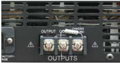
Figure B.2.38 – Output Terminal Resistor Location
