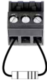
Figure B.2.22 – Terminating the Amplifier Input
