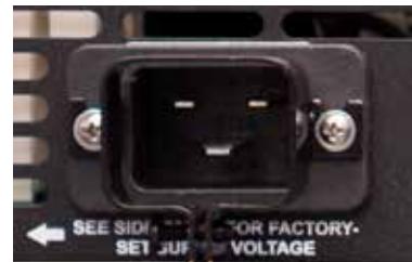
Figure 4.5 – Closeup of AC Mains Outlet
