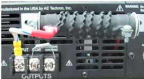
Figure B.2.18 – Connecting the Ballast Resistor
