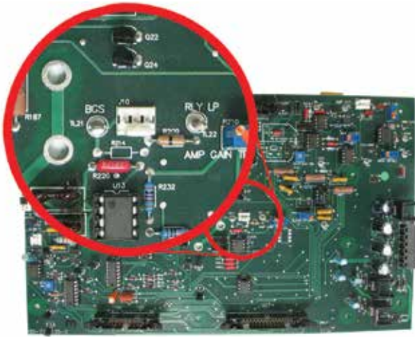
Figure B.1.3 – Configuring Fixed/Variable Gain
