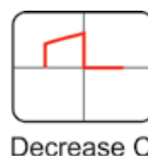
Figure 7.21 – Square Wave Showing a Decrease in C is Required
