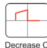
Figure B.2.8 – Square Wave Showing a Decrease in C is Required
