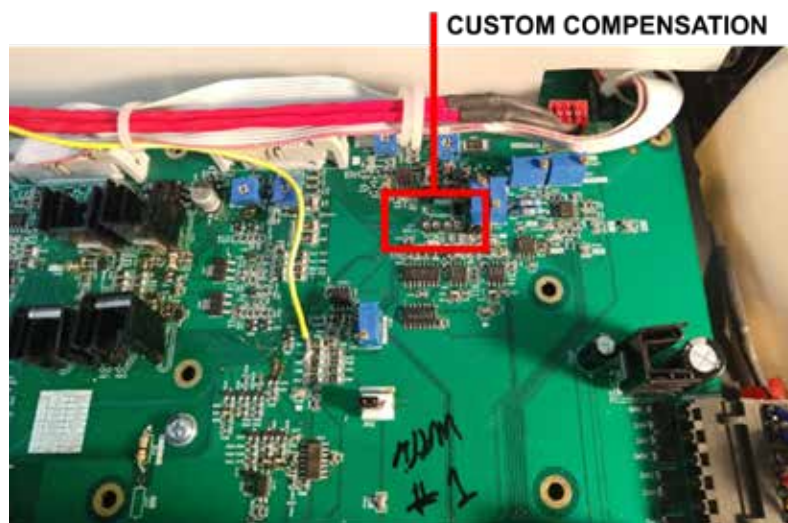
Figure 7.17 – Custom Compensation Component Locations
