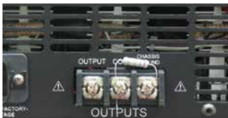
Figure B.2.38 – Output Terminal Resistor Location
