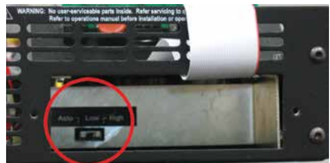
Figure 6.12 – Bi-Level Power Switch Location
