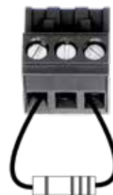
Figure B.2.39 – Terminating the Amplifier Input
