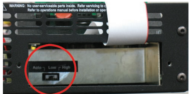
Figure 6.12 – Bi-Level Power Switch Location
