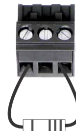
Figure B.2.11 – Input Terminator
