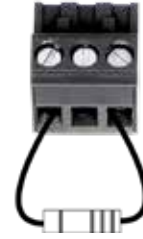
Figure 5.21 – Terminating the Amplifier Input
