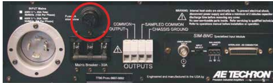
Figure 7.2 – Fuse F1 Location
