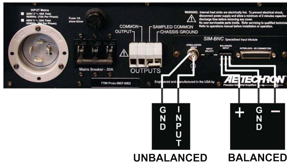
Figure 2.4 – Wiring for Unbalanced or Balanced Input Connector
