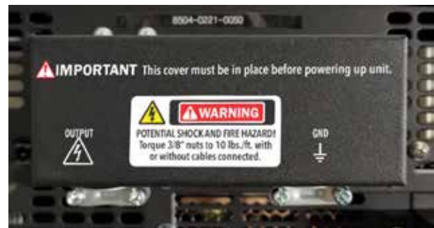
Figure 3.3 – Output Safety Cover
