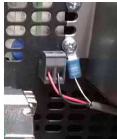
Figure 4.3 – Connected Remote Sense Port
