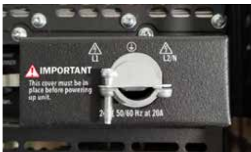
Figure 3.8 – AC Inlet Safety Cover
