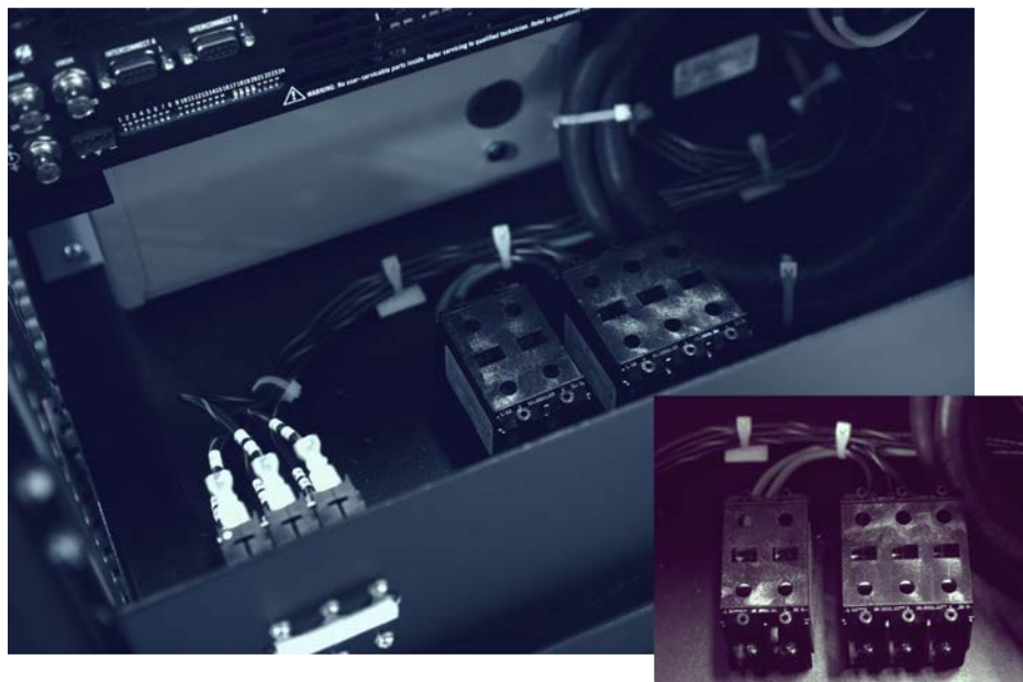
Figure 3.5 – Location of AC Mains Barrier Strip
