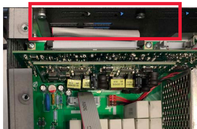
Figure 5.6 – Front-end board location
