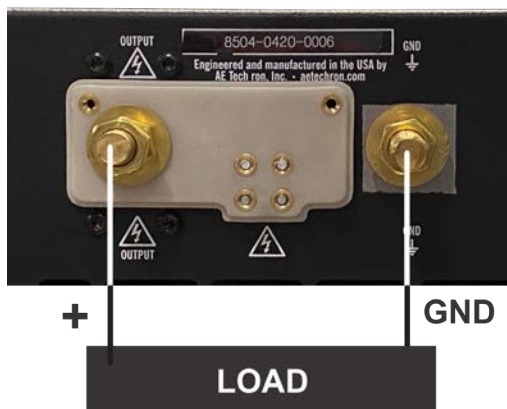
Figure 3.2 – Connecting the Load
