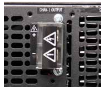
Figure 3.2 – Output Safety Cover
