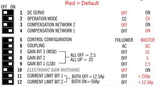
NOTE: GRAY TEXT INDICATES SWITCH USED FOR FACTORY CONFIGURATION ONLY. ALL BIT SWITCHES ARE ADDITIVE. RIGHT = <math>0N.
