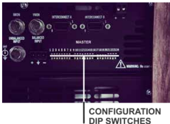
Figure 5.2 – DIP Switches Location on Master Amplifier Module
