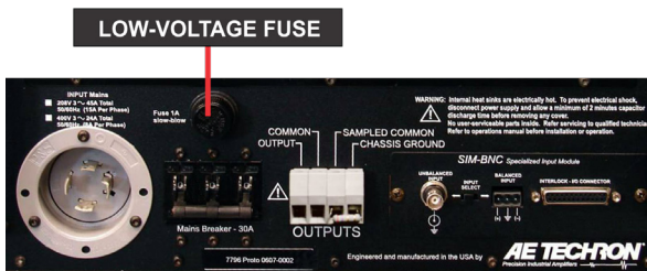
Figure 5.2 – Amplifier Module’s Low-voltage Fuse Location
