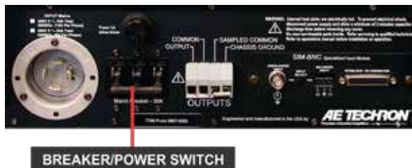
Figure 5.1 – Amplifier Module’s Breaker/Power Switch Location
