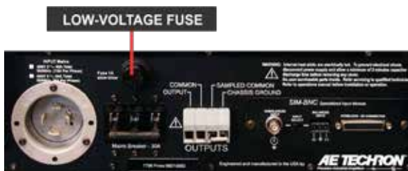
Figure 5.2 – Amplifier Module’s Low-voltage Fuse Location
