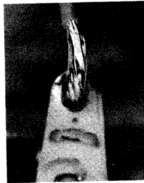
Fig. 7.8 Cold Solder Joint
