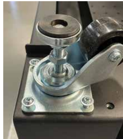
Figure 2.3 – Leveling pads on System's Wheels
