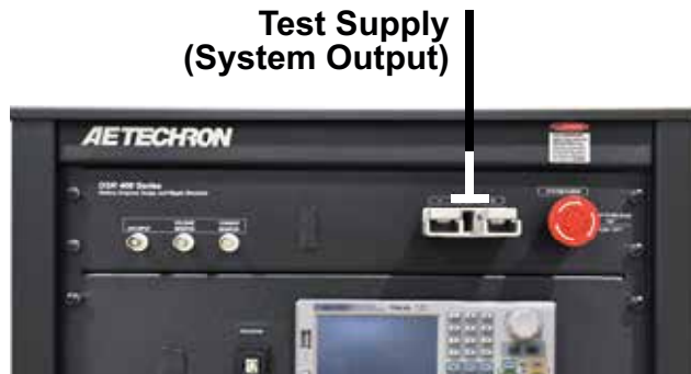
Figure 2.8 – Test Supply Connections (DSR 400 System Output)
