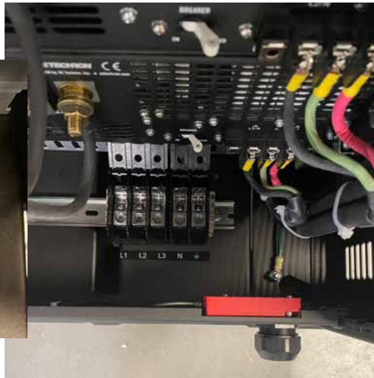
Figure 2.10 – Wiring the AC distribution block
