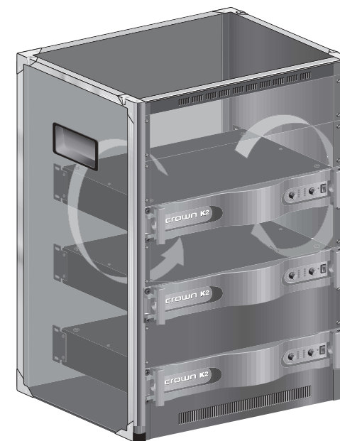
Figure 3.2 Spacing the Amplifiers in the Rack Improves Cooling
