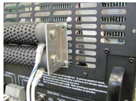
Figure 4.2 – 2120/7794/7796/7796HC Ballast Resistor Mounting
