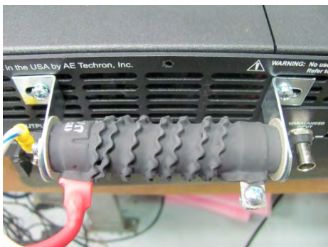
Figure 4.1 – 2105/7224 Ballast Resistor Mounting
