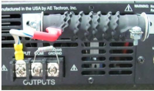
Figure 4.3 – 2105/7224 Ballast Resistor Connected to Output Terminal
