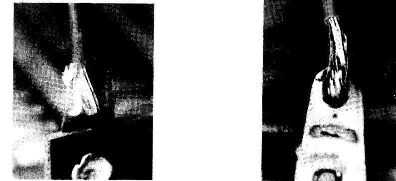
Fig. 7.8 Cold Solder Joint
