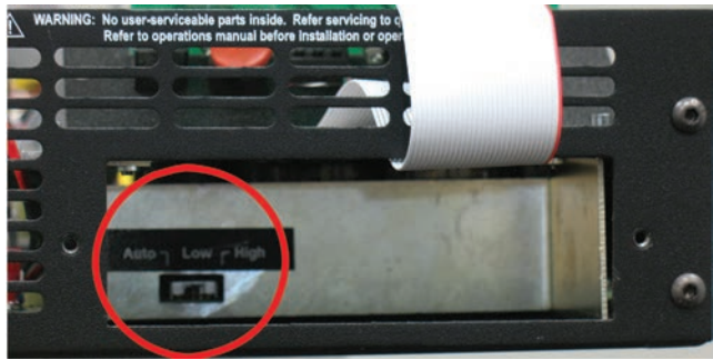
Figure 5.10 – Bi-Level Power Switch Location
