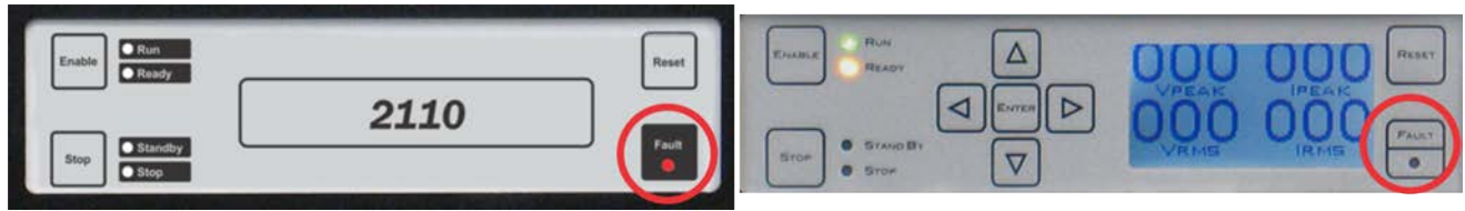
Figure 4.4 – Fault Status Indicators (2110 and 7794MRL models shown)
