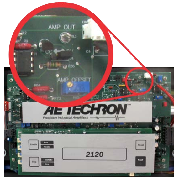
Figure 5.3 – Controlled-Voltage or Controlled-Current Mode Setting
