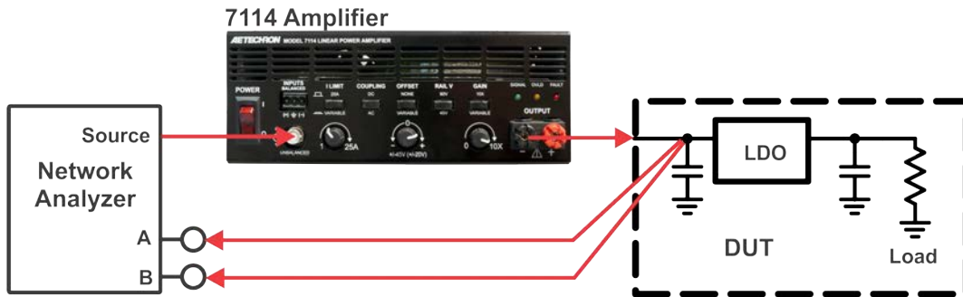
Figure 6.18 – LDO PSRR Measurement, Calibration Setup
