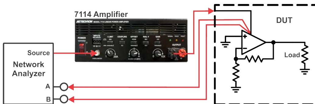
Figure 6.21 – Amplifier PSRR Measurement, Calibration Setup
