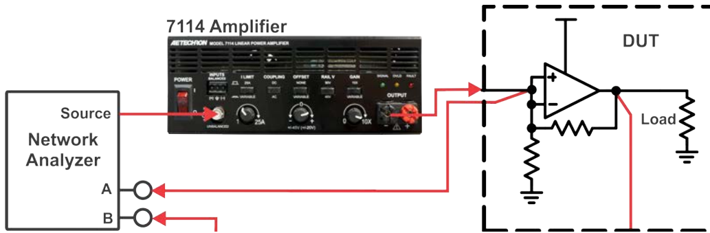
Figure 6.24 – Amplifier CMRR Measurement, Testing Setup
