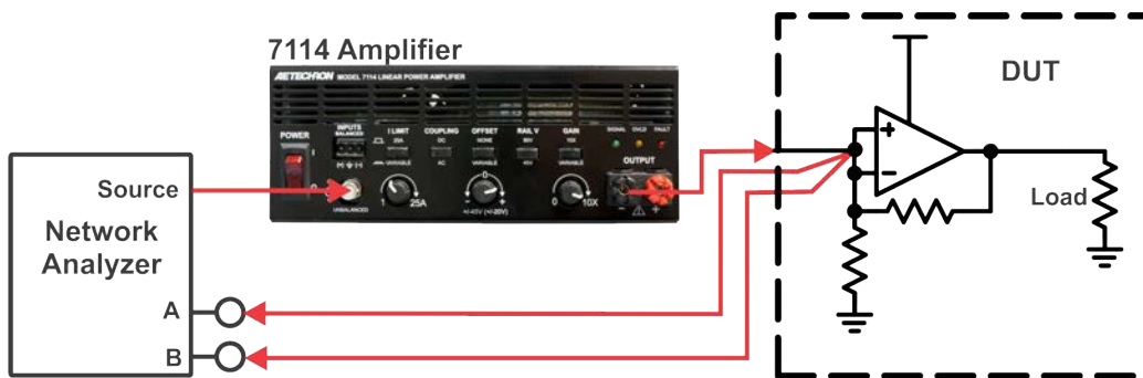
Figure 6.23 – Amplifier CMRR Measurement, Calibration Setup
