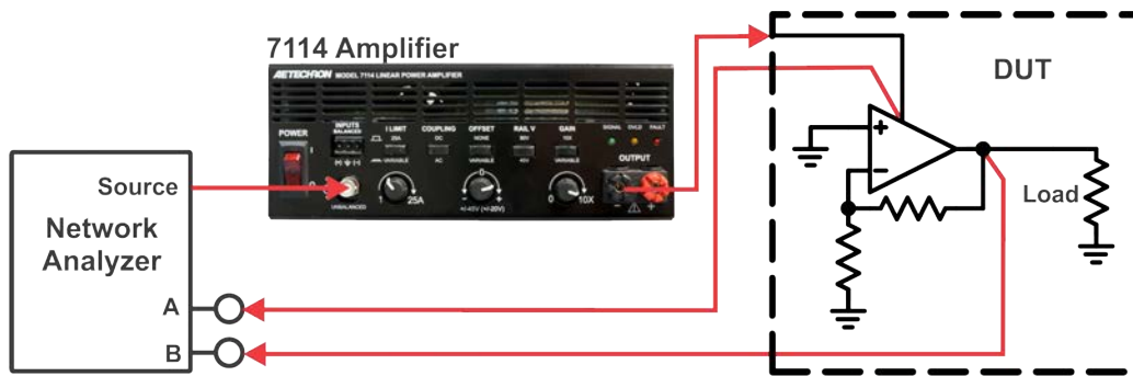
Figure 6.22 – Amplifier PSRR Measurement, Testing Setup
