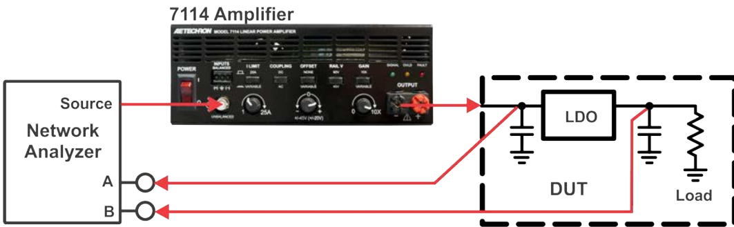
Figure 6.19 – LDO PSRR Measurement, Testing Setup
