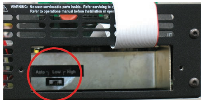
Figure 5.13 – Bi-Level Power Switch Location
