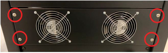
Figure 2.11 – Removing the fan panel
