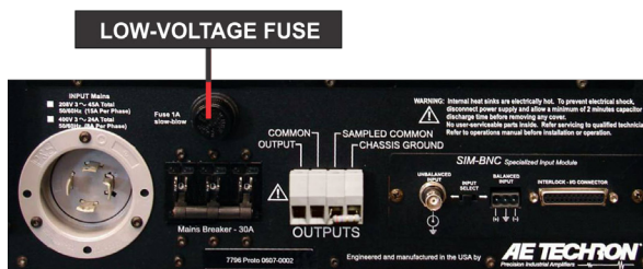
Figure 5.2 – Amplifier Module’s Low-voltage Fuse Location
