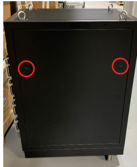
Figure 2.9 – Removing the right side panel
