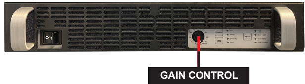
Figure 2.5 – Gain Control Location
