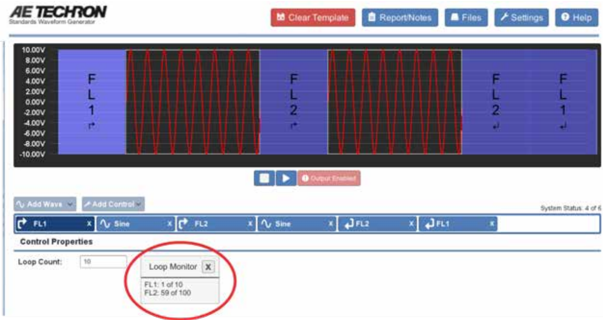
Figure 6.16 – Using the Loop Monitor
