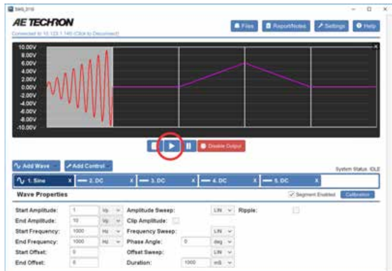
Figure 5.6 – Generating output signal
