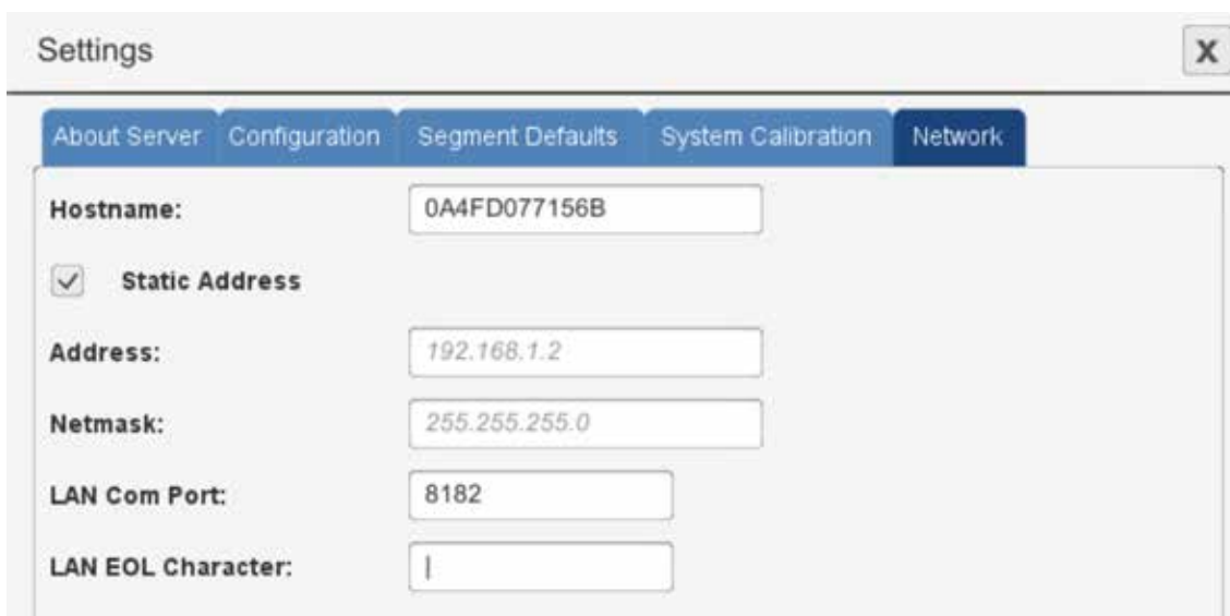
Figure 9.5 – The Network Tab in the Settings Window
