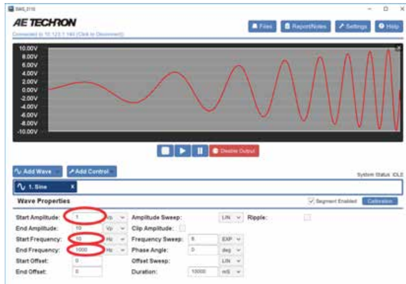
Figure 5.4 – Wave Properties window.
