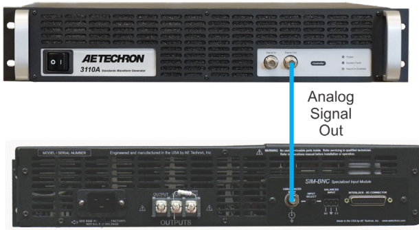
Figure 2.2 – Connecting an amplifier to the 3110A
