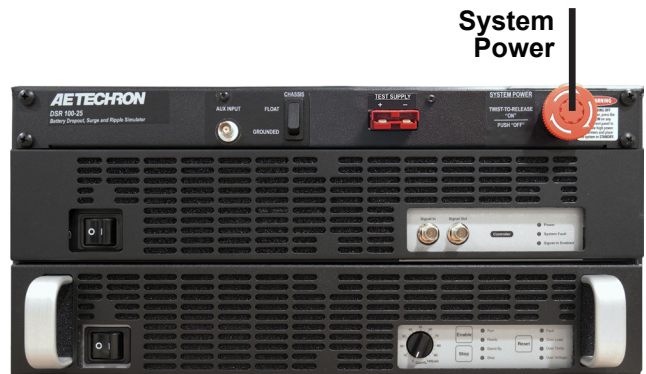
Figure 2.6 – System Power Switch Location
