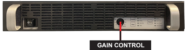
Figure 2.5 – Gain Control Location
