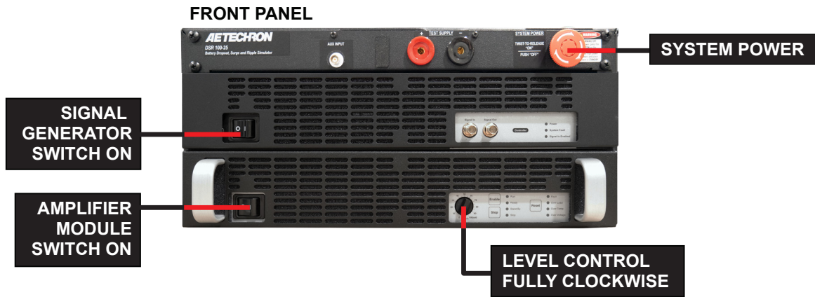
Figure 4.3 – Locations of Controls for Low-Voltage Testing
