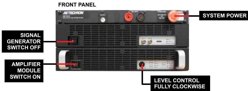
Figure 4.5 – Locations of Controls for Operation with an External Signal Source
