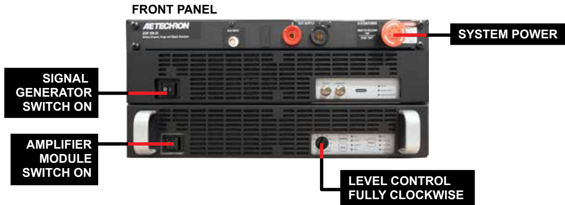
Figure 4.3 – Locations of Controls for Low-Voltage Testing
