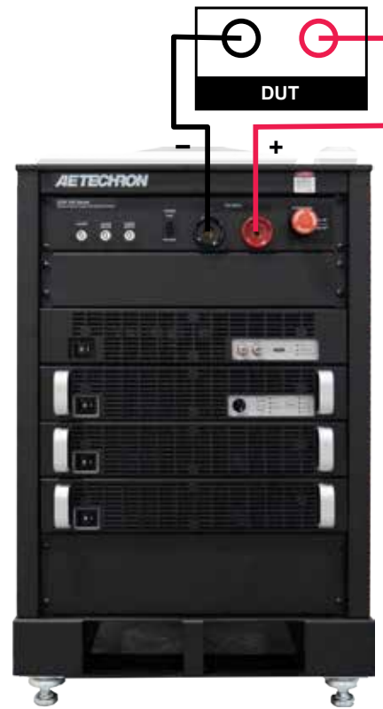
Figure 4.4 – Connections for Low-Voltage Testing
