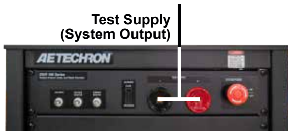
Figure 2.5 – Test Supply Connections (DSR 100 System Output)
