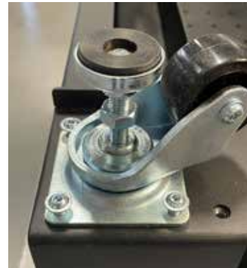
Figure 2.3 – Leveling pads on Wheels
