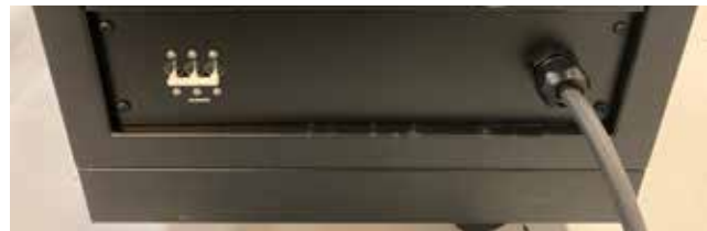
Figure 2.6 – Routing the AC power input cable
