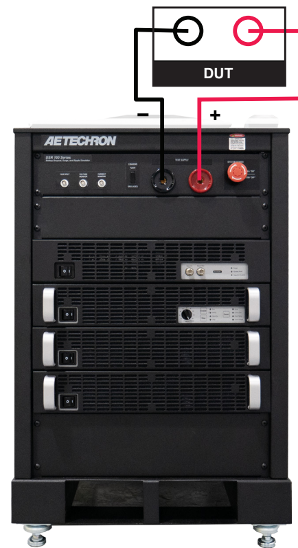
Figure 4.4 – Connections for Low-Voltage Testing
