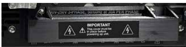
Figure 3.8 – AC Inlet Safety Cover
